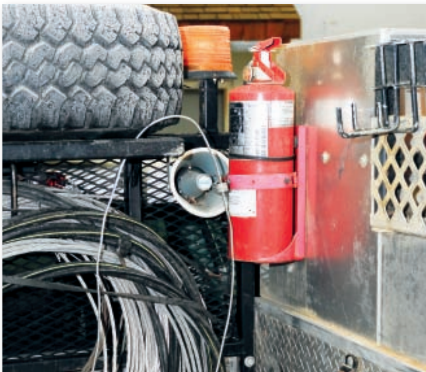
Mor-Gran-Sou's pick-up trucks carry one ABC, all-purpose fire extinguisher. The digger trucks carry two based on their size; one on each side of the truck for immediate access.
